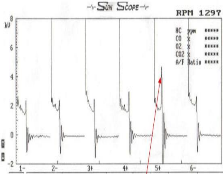
1997 Intrepid 3.5 with a P0305 DTC. Lean misfire caused by vacuum leak at #5 intake runner.
