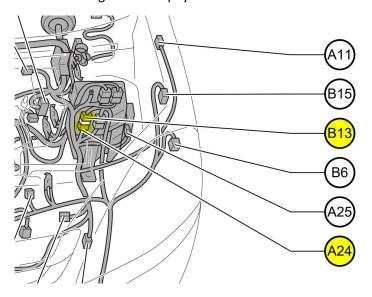
I disconnected B13 from the port in the fuse box. I also disconnected both 4A (Floor wire to the rear indicators) and 4B (Engine Room Main Wire) from the body control module.
