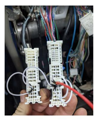
I must have checked the 4B connector pin 32 (Battery) to the front fuse over ten times with my multimeter, and I never found any resistance readings to ground. For this testing, the 4S connector was still connected to the body control module, but I had disconnected the headlamp dimmer switch, turn signal switch, combination meter (instrument cluster), and hazard light
