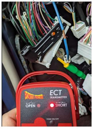
As a final step, I replaced the 4B pin 32 (Battery) wire with a new wire and jumped it directly to the other end of the "bridged fuse light" to rule out anything my multimeter might have missed. This also didn't solve the issue.
