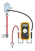
I checked each individual line (with the bulbs removed) for resistance readings to ground and found nothing. All lines appeared to be clear, with no resistance readings to ground. When testing the cables end to end, the resistance readings were fine, measuring less than 1 ohm.
