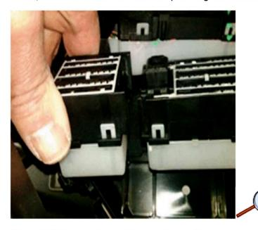
X1 and X3 Connectors slide together. Connectors must be fully seated.
