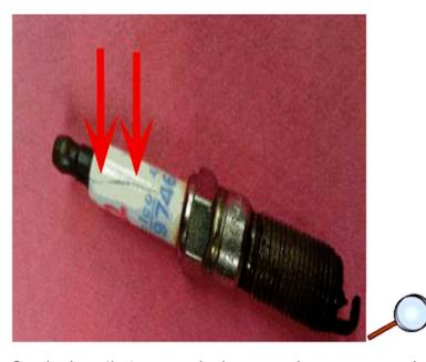
Spark plugs that are cracked, wrong plug gap, worn plugs, carbon fouling, and top post contact issues.
