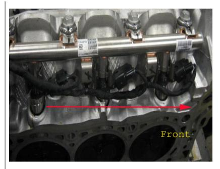
• Bank 2 injector connectors aim toward the front of the engine as shown above.
