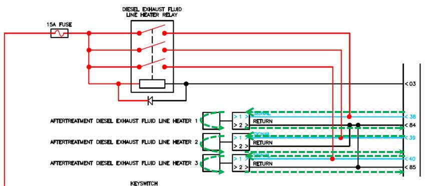
With 5 volts signal from ECM – Line heaters and ground wires verified for continuity at Key ON Expected Voltage drop between 38,39,40 and 84, 85 is 5 <u>Volts</u>
