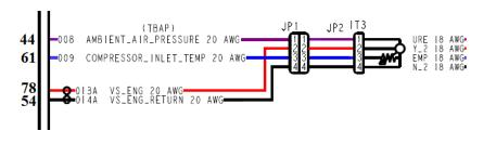
The turbocharger compressor intake temperature sensor is a variable resistor sensor and is used to measure the temperature of the air entering the compressor intake of the turbocharger. The electronic control module (ECM) supplies 5-VDC to the compressor intake temperature signal circuit. This sensor signal voltage changes, based on the pressure in the intake manifold.
