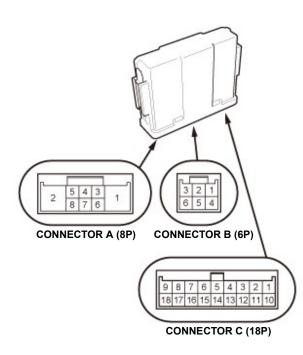
The relay circuit board is part of the under-hood fuse/relay box and contains these relay circuits:
