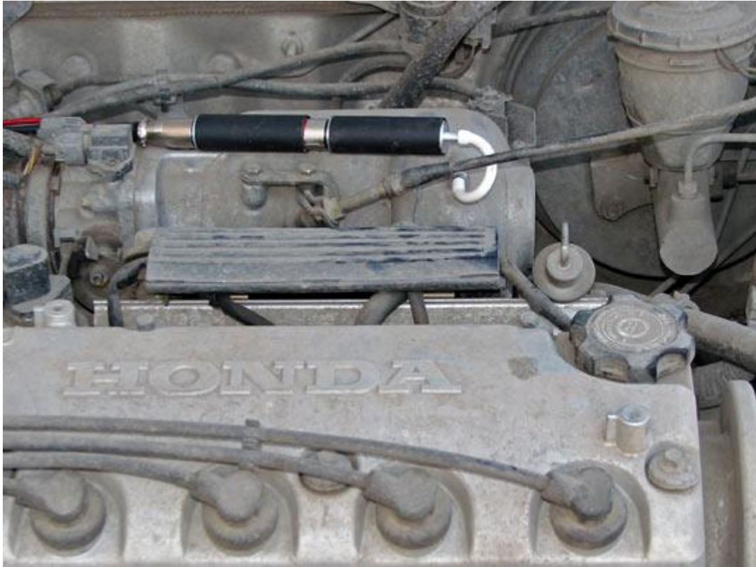
The low pressure transducer Dx with Dx Amplifier is connected to the intake manifold using a short vacuum tube.
